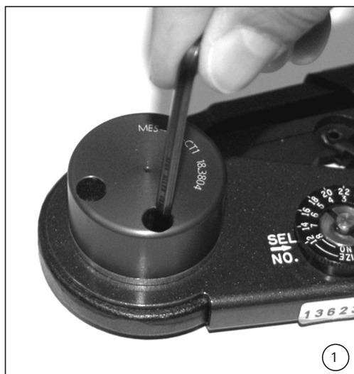
(ill. 1) Locator befestigen mittels mitgeliefertem 6-kant Schlüssel.
